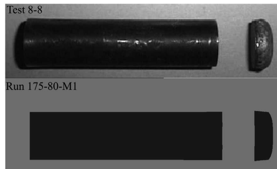
Fig. 12. Projectile and plug after perforation (test 8-8 and Run 175-80-M1).
